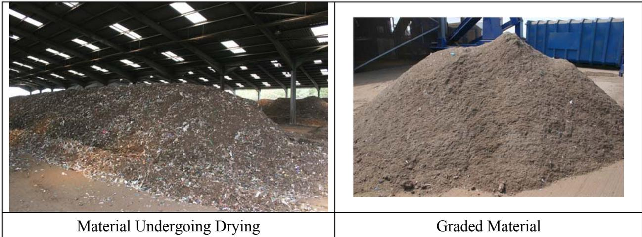
**Figure 2 Comparison of G2S Graded and Ungraded Material**
