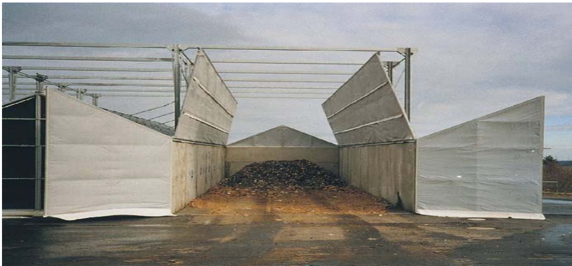
Figure 3 Typical in-vessel composting clamp
